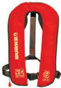
The lifejacket is manually inflatable by pulling the toggle on the lower right side of the jacket. This action punctures a CO2 cylinder inside the jacket inflating it. They are suitable for anyone over 40kg in body weight.
